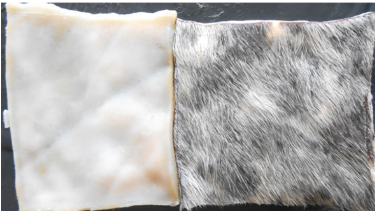
Fig. 3 Photograph of hide completely dehaired by crude alkaline protease within 3 h (pH 12 and 37°C); negative control where distilled water under the same condition remained with hair
