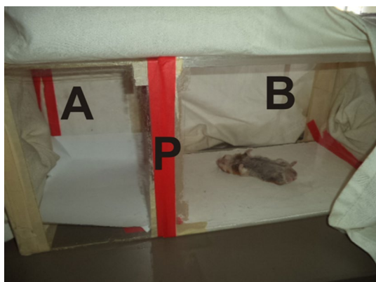
Fig. 1 Perspex cage measuring 25 X 25 x 80 cm (length) separated by a removable cardboard frame (P). The restrained hamster smeared with the oil preparation on the legs, tail, and mouth parts is on the test chamber B. Sand flies were held in chamber A and had to make contact with the removable cardboard and pass through the perforated partition (P) to reach the bait (hamster) in chamber B. Repellency was determined by counting the number of sand flies that landed on the hamsters' legs, tail, and mouth parts for a period of five minutes each at intervals of 30 min
