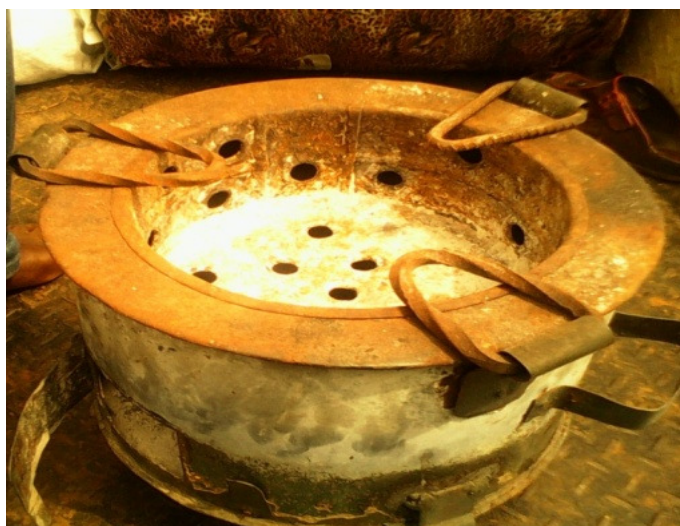
Figure-5 Improved metallic cookstove based
