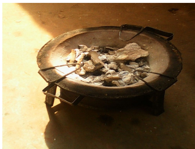
Figure-6 Improved Cookstove with Inner Lining
