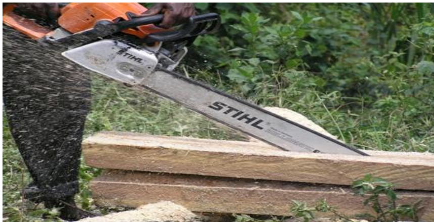
Plate 2.3: A Chainsaw Converting a Log into Lumber (Wood-mizer, 2018)
